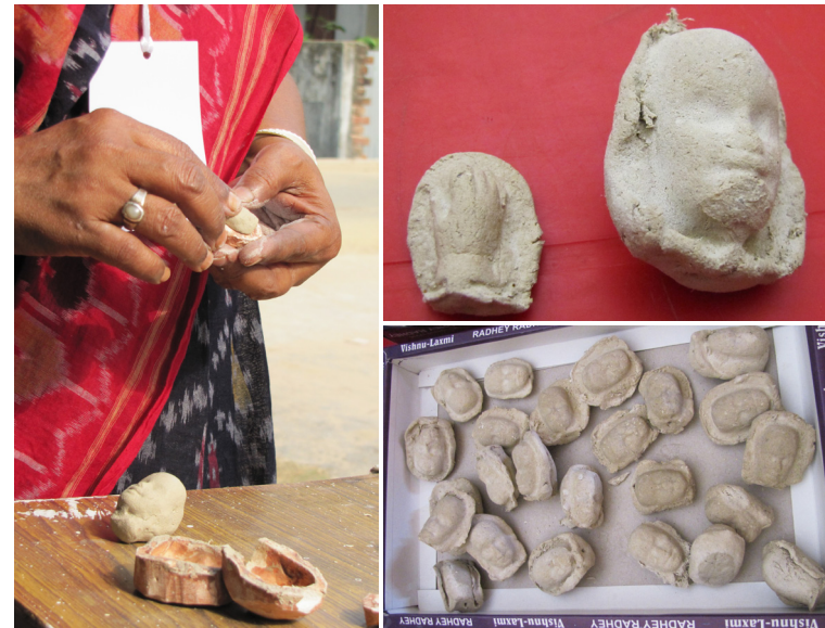
Making head - hands - feet using dies
